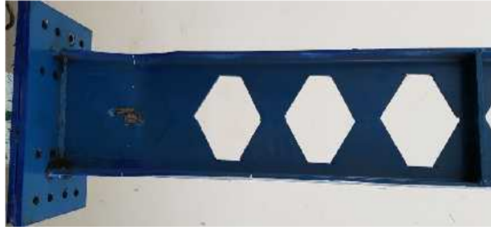
Figure 7. Damage on the specimen that was subjected to cyclic loading.
